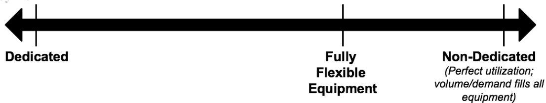
Fig. 5. This chart illustrates the spectrum of dedication on the line. Equipment dedication to the line, including specialized designs requiring unique equipment dedication, fall on the left; non-dedication (indicating perfect utilization of the equipment) on the right. Fully flexible equipment would allow products to share equipment, reducing the utilization impacts of dedication. In our case, flexible equipment leads to an approximately 4% reduction in cost for a mix of all products in the extreme case, and full non-dedication amounts to an approximately 5% cost reduction for the same mix.
